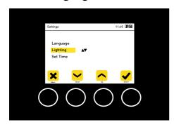
When pressing the *Settings* button in the main menu, the language, illumination, and time screen opens. The arrow keys allow you to make a selection, and choosing the *Select* function takes you to the various options. These, in turn, can also be selected by activating the arrow keys. Acknowledge your selection by pressing the *Select* button. Press the *Abbort* button to return to the main menu.
