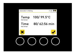
As described in the previous section, automatic brewing continues and the hops boiling process is started. The display again shows the time and temperature of the phase. As the target temperature of 100°C cannot always be reached, timing starts after a waiting period of 2 minutes without increase in temperature. When pressing the *Select* button during the automatic mode, the target temperature and target time can be corrected or changed. Wort is boiled during this phase. On the one hand,
