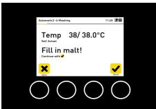
When reaching the mashing-in temperature, a signal will be sounded and the lights will be blinking. This must be acknowledged by pressing the *Select* button. This switches the pump off. Now, follow the instructions of the brew control.
