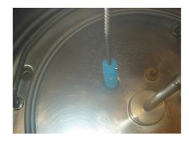
Basic cleaning also includes cleaning of the suction and pressure openings.
