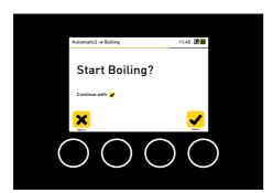
After removing the malt pipe, acknowledge it by pressing the *Select* button. In order to start the hops boiling process, press the *Select* button again. The pump and the heating switch on again and the automatic process continues.
