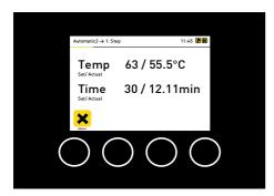
The display now indicates the rest, target, and actual temperature, and the target and actual time. After the target temperature has been reached, the countdown starts. All other phases are processed fully automatically. The display indicates in the respective times and temperatures.
