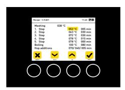
Plug in the Braumeister. The control is now in a basic state. In order to program a recipe, its time and temperature values, press the *Recipe* button. Use the arrow keys in the menu display above to select the recipe with which you would like to work. you can also create new recipes (up to 10) or delete recipes. Two standard recipes are included with the delivery. Press *Select* to invoke the recipe. Continue pressing *Select* while in the recipe step by step until you reach the end.
