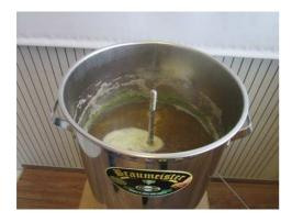
Continue by pressing the *Select* button in order to start the hops boiling process. Do not close the lid. Avoid the hops boiling over. Add the first hops batches of 10 g / 20 g/ 50 g 10 min after the boiling process has started. Do not close the lid during the hops boiling process either. Steam must be able to escape. Top up evaporated water quantity or adjust original wort. Add the last batch of hops 10 min before end of boiling.
